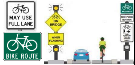
"Bikes on Bridge" activated warning.
