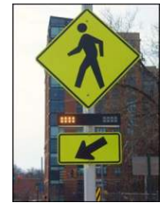
Rapid Rectangular Flashing Beacon (RRFB)
