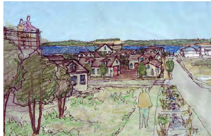
Rendering from the same angle showing how the view would be opened up by laying back the slope. Note bioswale treatment to manage stormwater runoff.
